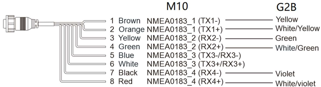
Figure 64 - Wiring connection between G2B and M10.
